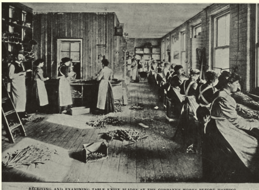
RECEIVING AND EXAMINING TABLE KNIFE BLADES AT THE COMPANY'S WORKS REFOR HATTING.
